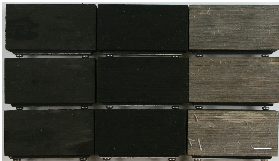
Fig. 1 Oil-treated pine sapwood samples with natural formed biofinish and weathered samples without biofinish. Samples in the left row : treated with raw linseed oil. Samples in the middle row : treated with olive oil. Samples in the right row : untreated. Scale bar 10 mm
