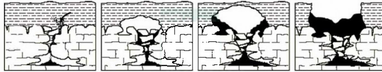
Formation of a Collapse Sink
