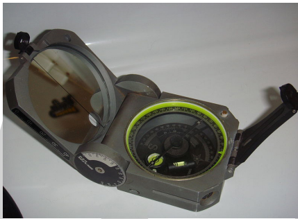
A standard Brunton Geo compass, still used commonly today by geographers, geologists and surveyors for field-based measurements.
