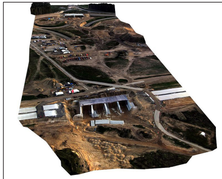
Digital Surface Model of motorway interchange construction site. Note that tunnels are closed.
