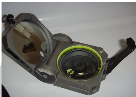
A standard Brunton Pocket Transit, commonly used by geologists for mapping and surveying.
