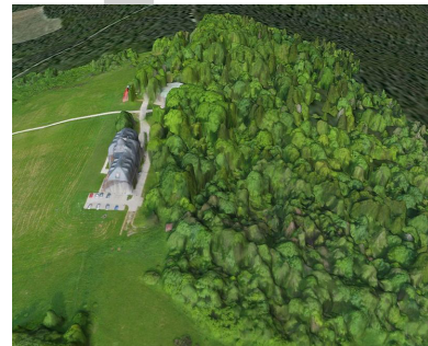
Bezmiechowa airfield 3D Digital Surface Model obtained using Pteryx UAV flying 200 m above hilltop.
