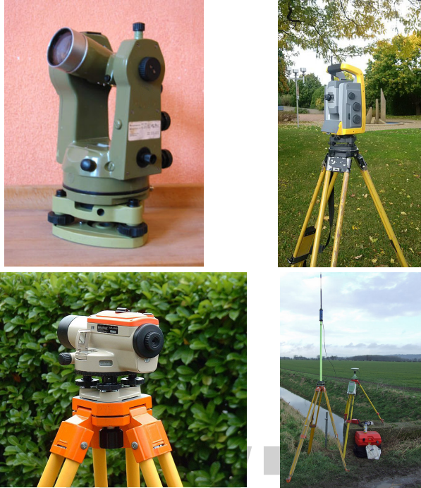
Surveying equipment. Clockwise from upper left: optical theodolite, robotic total station, RTK GPS base station, optical level.
