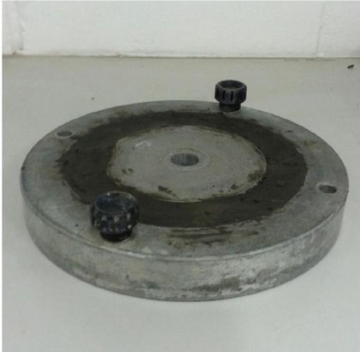
Figure 2. Sample prepared before the consolidation stage.
