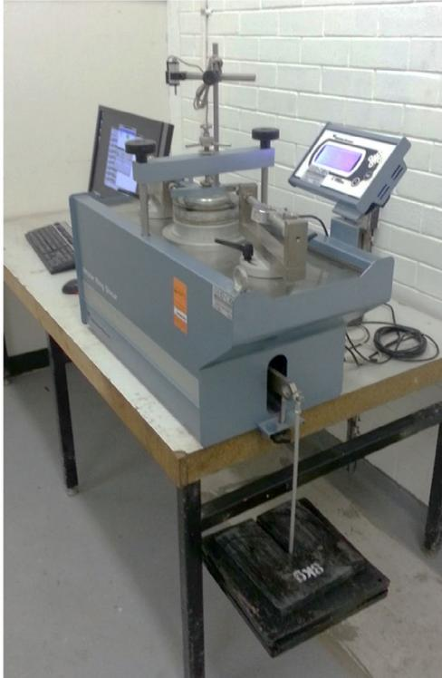
**Figure 1. Ring shear apparatus used in this study.**
