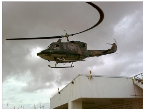
Distortion caused by a rolling shutter.
