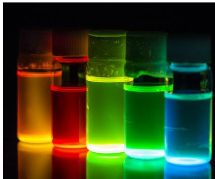
Colloidal quantum dots irradiated with a UV light. Different sized quantum dots emit different color light due to quantum confinement.
