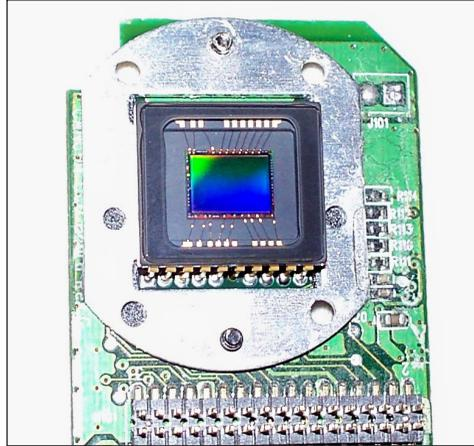
CCD from a 2.1 megapixel Hewlett-Packard digital camera.
