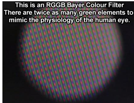
x80 microscope view of an RGGB Bayer filter on a 240 line Sony CCD PAL Camcorder CCD sensor.
