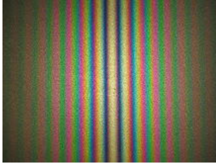
Fringe pattern produced with a Michelson interferometer using white light. As configured here, the central fringe is white rather than black.
