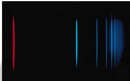
The Balmer series of hydrogen as seen by a low-resolution spectrometer.
