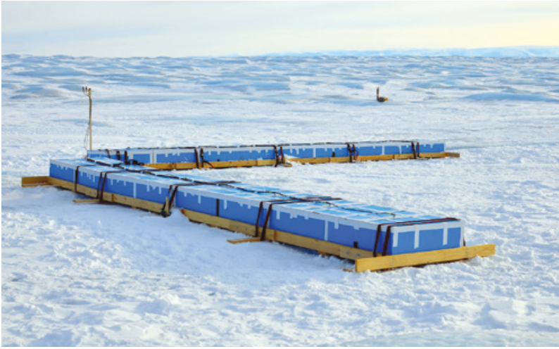
Fig. 4.4 Photograph of the experimental imaging radar deployed on Store Glacier in 2014 (Photo: T. J. Young).
